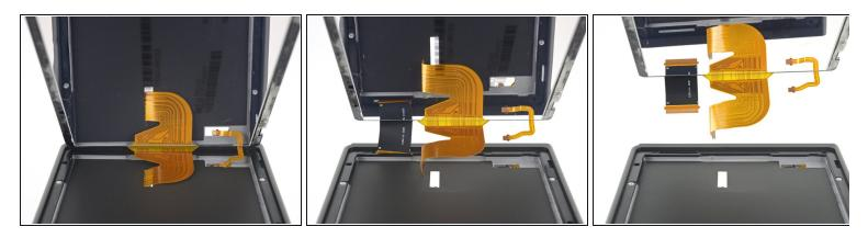
• Lift the right edge of the screen straight off the device, threading the ribbon cables through the frame as you do so.
