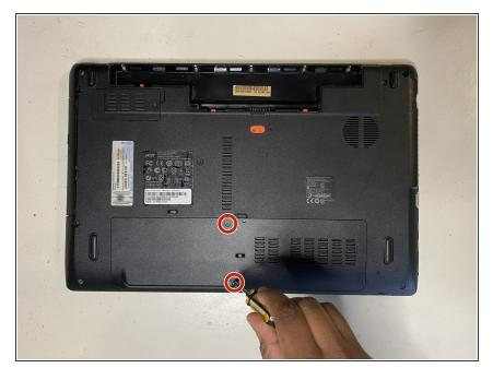
Remove the two M2.5X8 screws using the Phillips #0 screwdriver.
