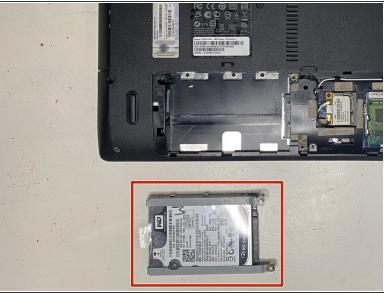
Pull the tab and lift up to remove the hard drive.
