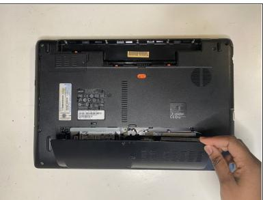
Remove the cover to access the hard drive.
