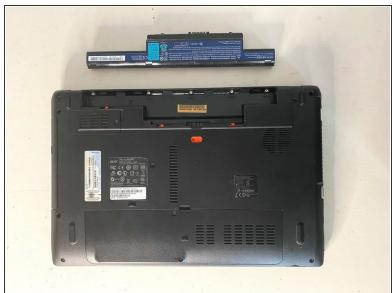
Slide the battery out and remove it.
