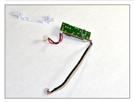
Separate the white suport bracket from the headphone/power electronics board.
