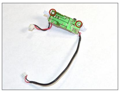
Unscrew the two 5 mm Phillips #00 screws from green Headphone/Power electronics board to detach from white support bracket.
