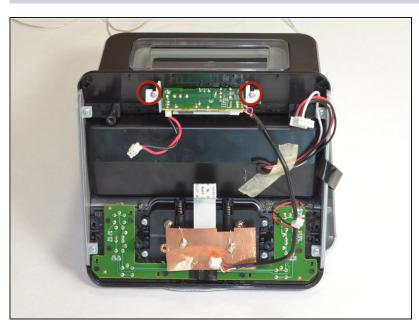
Unscrew the two 5 mm Phillips #00 screws attaching white support bracket to the body of the device.
