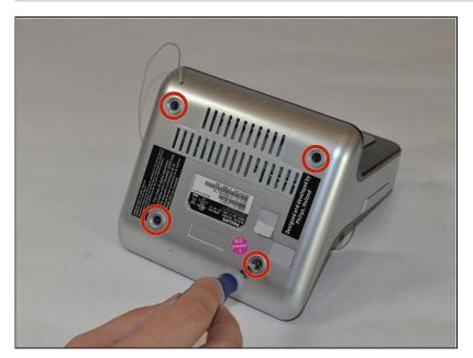
Gently unscrew the four 15.5 mm Phillips #2 screws that hold the bottom panel to the dock.
