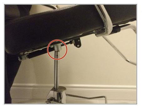
Align the bottom of the seat with the top of the pole, and gently put it back into position.
