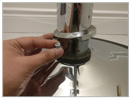
• Lift the base-ring off the base to reveal the holes for the screws.
