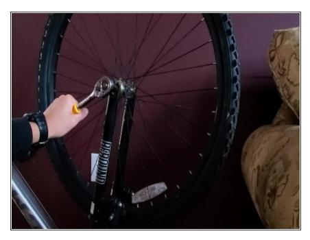
Using a torque wrench with the 15mm socket, loosen the two bolts on the axle that keep the tire in place.
