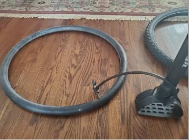
Using the bike pump, inflate the new inner tube until it becomes circular.
