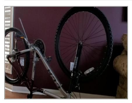
Pull the tire in an upward motion, releasing it from the brakes and axle.
