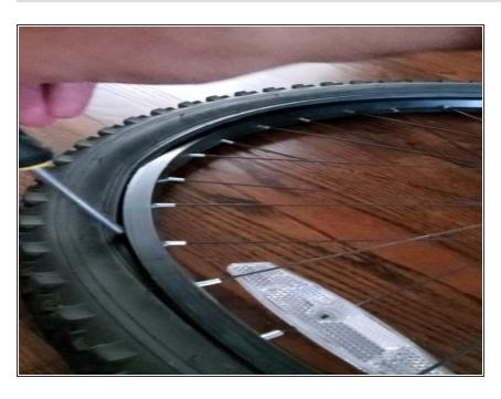
Insert a prying tool in between the tire and metal rim and push it outward, dislodging it from the rim and making it easier to remove.
