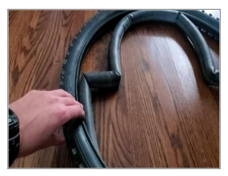
Place the new inner tube inside the inner section of the outer tire.
