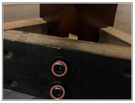
• Use an electric drill or a screwdriver to tighten the screws.
