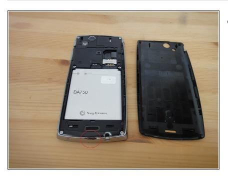
Start by removing the back cover, by inserting thumb nail into the slot and prying it open
