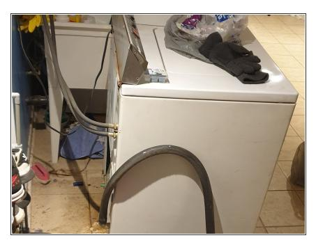
Adjust the washing machine to make enough space to walk in and clean the drain hose.
