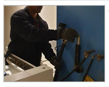
carefully attach the drain hose back.
