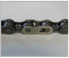
Hold the chain on either side of the master link, and pull them apart. The master link will snap
