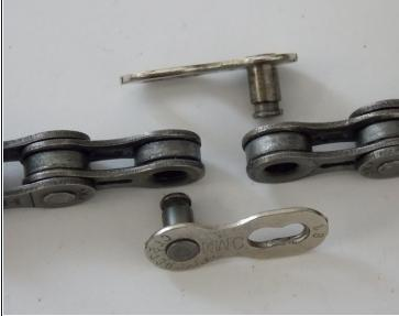
Slot the two halves of the master link together. One half's pin should go in the other's hole, and vice versa.
