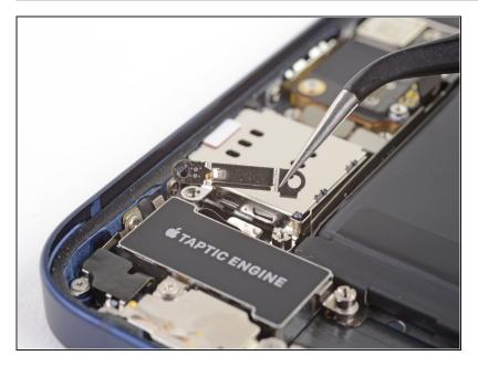
Remove the Taptic Engine cable connector bracket.
