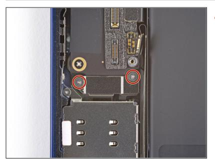
Use a Y000 driver to remove the two 1.4 mm long screws securing the SIM card reader connector cover.
