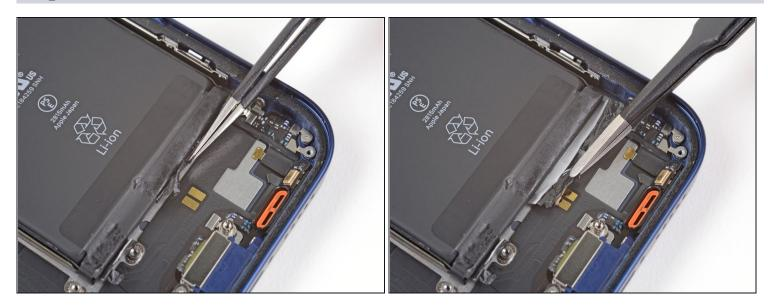
Peel down the second battery adhesive pull-tab to un-stick it from the bottom edge of the battery.
