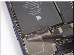
Peel up the two remaining battery adhesive pull-tabs to un-stick them from the top edge of the battery.
