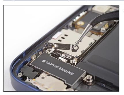
Remove the Taptic Engine cable connector bracket.
