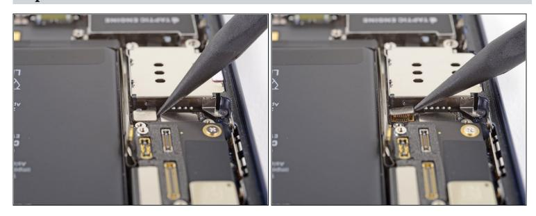
• Use the point of a spudger to pry the SIM card reader cable connector straight up and out of its socket on the logic board.
