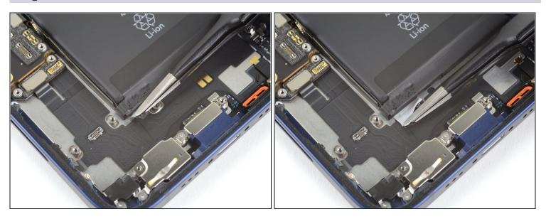
• Peel down the first battery adhesive pull-tab to un-stick it from the bottom edge of the battery.
