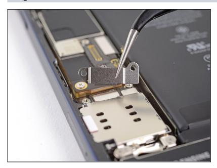
Remove the SIM card reader cable connector cover.
