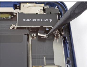
Use the point of a spudger to pry the Taptic Engine cable connector straight up and out of its socket on the logic board.
