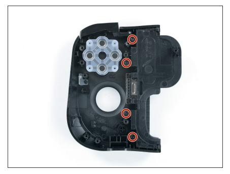
Use a Phillips #00 screwdriver to remove the four 5.7 mm screws securing the phone bracket.
