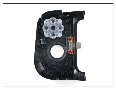
Use a Phillips #00 screwdriver to remove the two 4.6 mm screws securing the phone connector.
