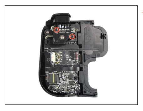
Use a Phillips #0 screwdriver to remove the two 4.4 mm-long screws securing the trigger board.
