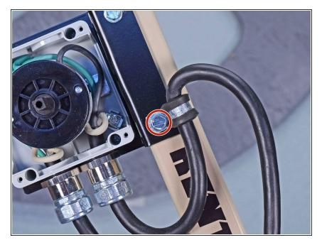
Use a 3/8 inch socket to remove the bolt securing the power cord loom clamp to the switch bracket.
