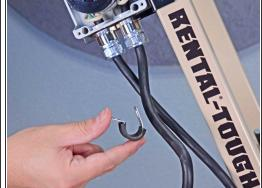
Remove the loom clamp from the power cable.
