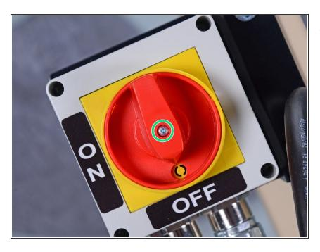
Use a Phillips screwdriver to remove the screw from the center of the red on/off knob.
