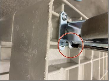
• Use the Phillips #2 screwdriver to remove all the screws from the metal plate.
