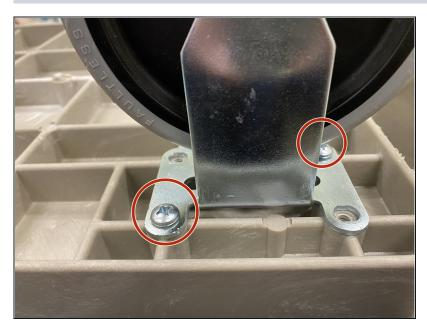
With the Phillips #2 screwdriver, secure the screws back in diagonally.
