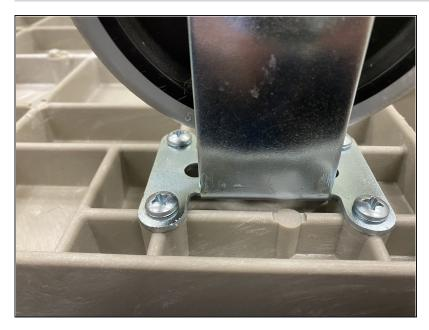
• Insert and secure the other two screws.
