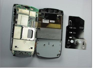
• Slide the slim metal plate upwards until it disconnects from the motherboard.
