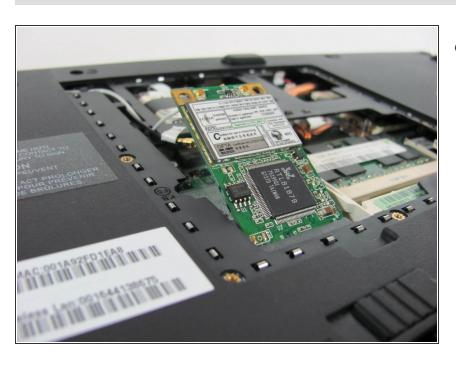
The wireless card will automatically pop up allowing for easy removal.
