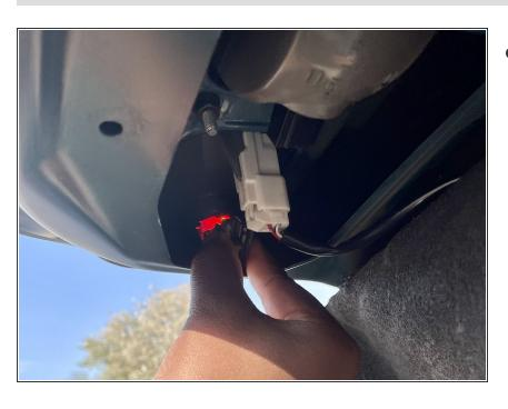
Repeat this process with the outer light bulb assembly using bulb 904.
