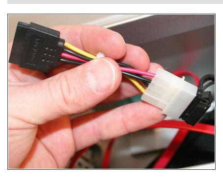
Connect the power converter cable to the already provided secondary power connector.
