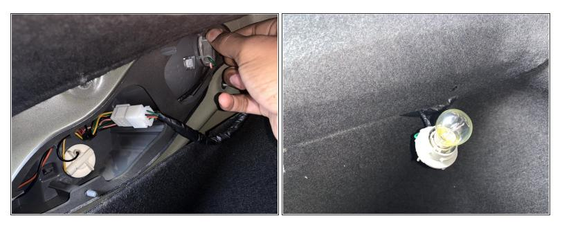
• Twist the socket counterclockwise to gain access to the brake light.
