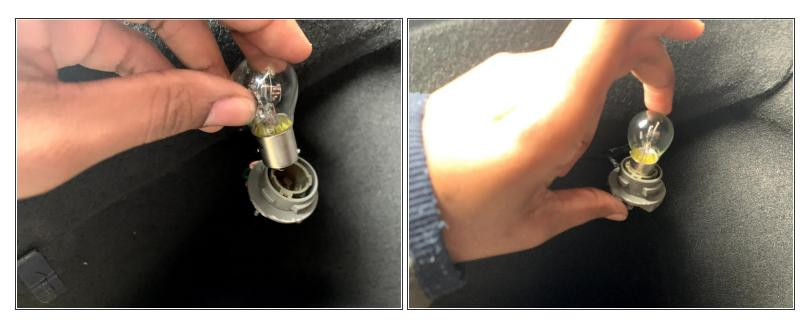
• Insert the new bulb into the socket and twist the bulb clockwise to secure it into place.
