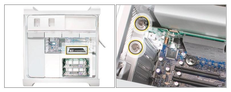
• This procedure explains how to remove a standard card and a card that includes a booster cable. Before you can remove either type of card, however, you must first loosen the two captive screws that secure the PCI bracket to the enclosure and remove the bracket.
