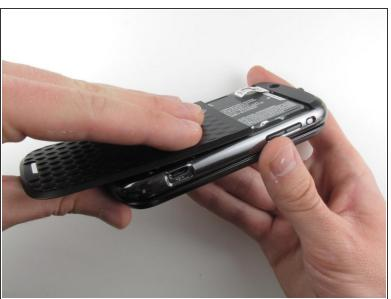
Turning over your phone, place two fingers on the back cover and apply pressure away from the camera to slide the back cover off.
