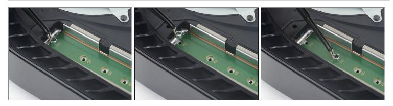
• Use a pair of <u>tweezers</u> to lift and move the spacer to the appropriate slot for your chosen M.2 SSD.
