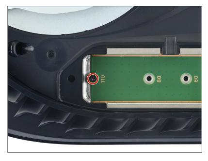
Use a Phillips screwdriver to remove the 11 mm-long SSD screw.
