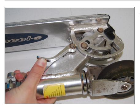
Start by pressing the lock lever with your thumb and unfold the scooter into riding position.
