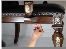
Tighten up the screw with a hex wrench screwdriver.
