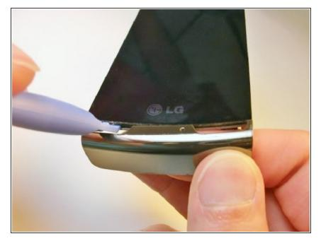
Wedge the plastic opening tool under the screen where the buttons were to loosen it.
