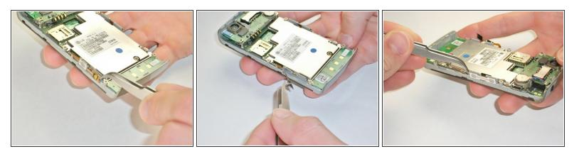
Use the metal tweezers to gently peel the yellow tab from the left edge of the phone at the two plastic bases.
