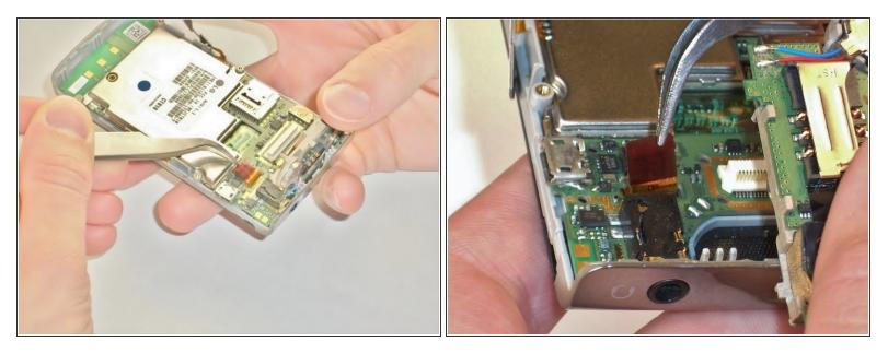
• Use the metal tweezers to gently lift the edge of the maroon tab, it should pop up easily.
