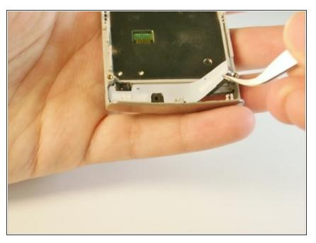
• Remove the call and end buttons using the metal tweezers.
