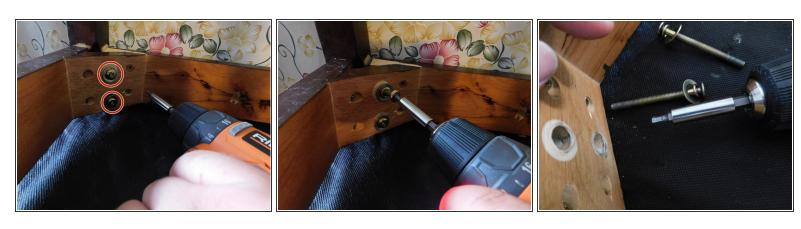
Use a power drill with a hex bit to remove the screws.
