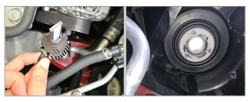
Align the three tabs on the new bulb to the three spaces in the housing for the headlight bulb.
