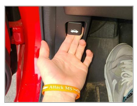
Pull the latch near the door panel to open the hood (inside the driver's side of the vehicle).
