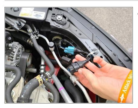
Reconnect wires to the new bulb.
