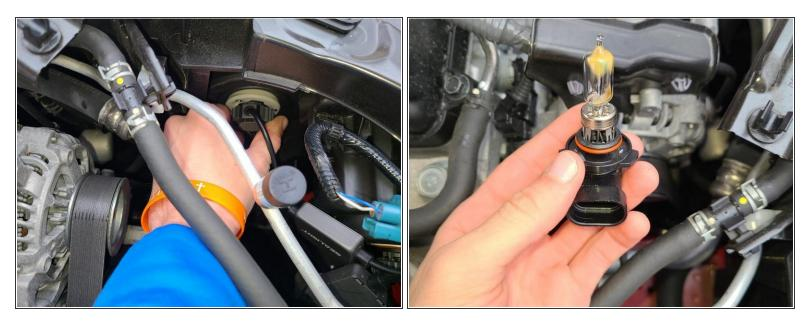
Twist the bulb counterclockwise and pull bulb out.
