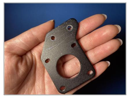
Buy a new bracket with the same brand (depending on the severity of the bend of the bracket) or straighten the metal on your own.
