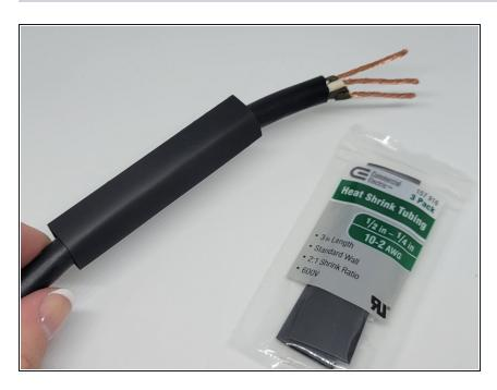
Before attempting to work with the wires, insert the cord into a piece of heat shrink tubing. This will help to safely seal the wires later.
