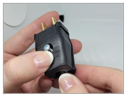
Unscrew the hinge on the new plug, set the screw somewhere safe for later.
