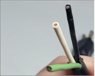
• Examine the 3 wires inside. You should see green, white, and black. Snip off any stray wires over a trash can.
