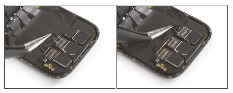
Use a pair of tweezers to carefully peel off the tape covering the middle and left display cable connector.
