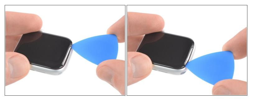
Slide the opening pick around the corner to cut the remaining adhesive on the short edge farthest away from the crown.
