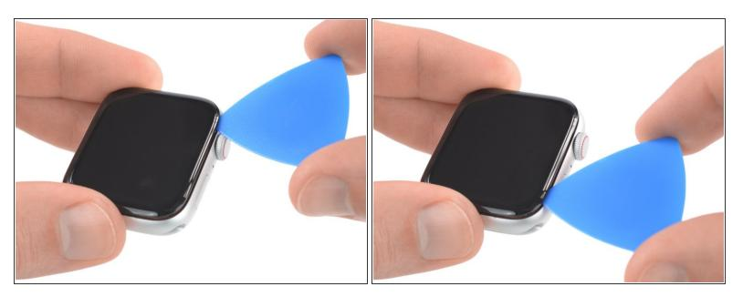
Mhen slicing near the crown, don't insert the opening pick deeper than 1/16th of an inch (~2 mm).
