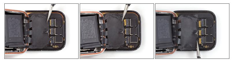
• Carefully pull the display flex cables out of their ZIF connectors.
