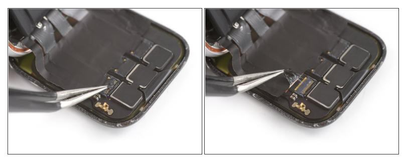
• Use a pair of tweezers to carefully peel off the tape covering the right display cable connector.
