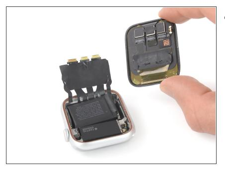
• Separate the watch assembly and the display.
