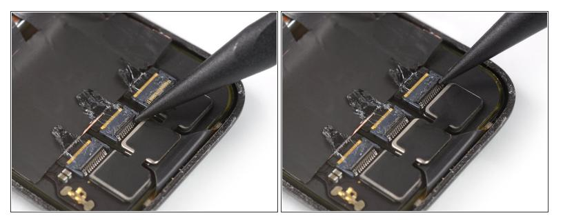
Use the pointed end of a spudger to open the middle and left ZIF connectors by bringing their flaps to an upright position.
