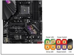
Plug the Power Led + into the top left prong. Positive goes on the left prong.
