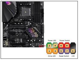
Plug the Power SW cable in above the Reset SW on the motherboard. This will allow you to turn
