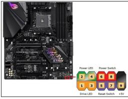
Plug the cable marked Reset SW into the motherboard. This will allow your reset button to actually work.
