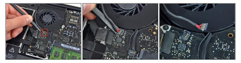
• Use the flat end of a spudger to pry the subwoofer/right speaker cable connector up off its socket on the logic board.
