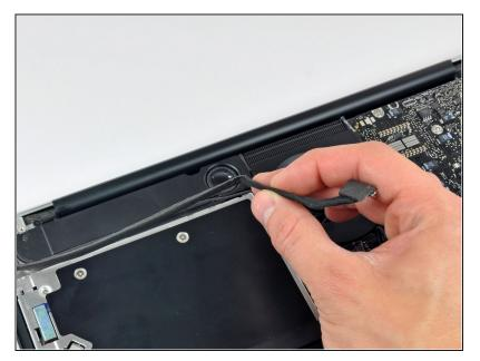
• De-route the camera data cable from the channel in the optical drive.
