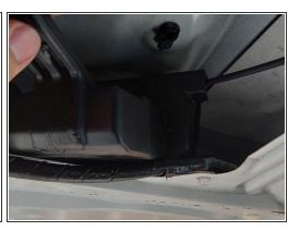
Using your hands, slide the trunk latch to the right side of the trunk and remove.
