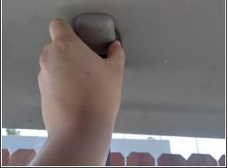
Pull upwards on the plastic covering the trunk strap to remove it.
