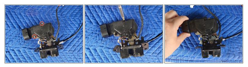
• Use a Phillips screwdriver to remove the two screws holding the actuator motor to the trunk latch.
