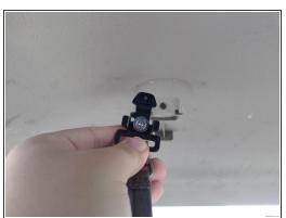
Using a Phillips screwdriver, remove the screw holding the trunk strap.
