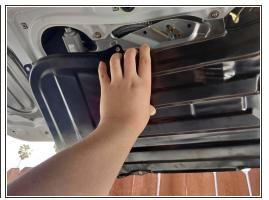
Use a spudger to partially pry open the plastic discs holding the metal trunk cover and push the trunk cover off the discs.
