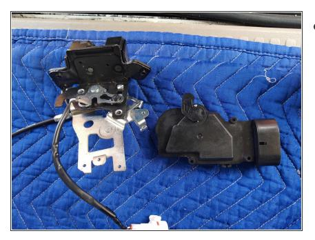
You can now reuse or replace your old actuator motor and attach it to a new liftgate latch.
