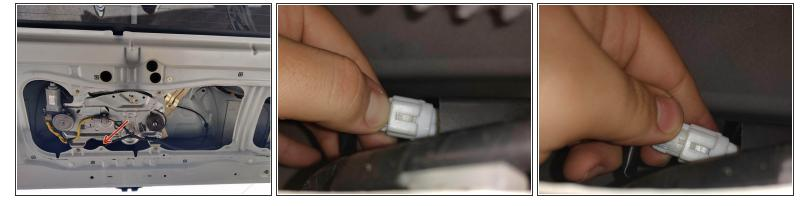
Use a flashlight and your hands to squeeze to remove white plastic plug connected to the trunk latch.
