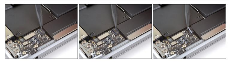
Slide the pointed end of a spudger underneath the speaker cable and pry straight up to disconnect it.
