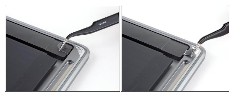
• Use a pair of tweezers to peel back the black pull tab on the speaker's stretch-release adhesive until you can grip it with your fingers.
