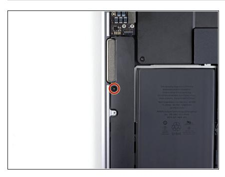
Use a T3 Torx driver to remove the 4.2 mm screw securing the right speaker to the case.
