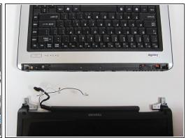
• Carefully pull apart the LCD display from the base by pulling vertically upwards on the display.
