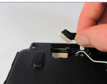
Disconnect the video cable connecting the display to the base of the laptop.
