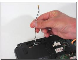
• Unwind the wires from the plastic tabs holding the wires in place.
