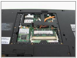
• Use a finger to remove the panel by lifting up on the provided removal tab.
