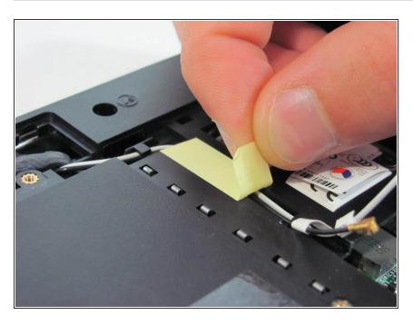
Remove the yellow tape holding the black and the white wires in place.
