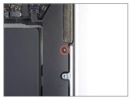
Use a T3 Torx driver to remove the 4.2 mm screw securing the left speaker to the case.
