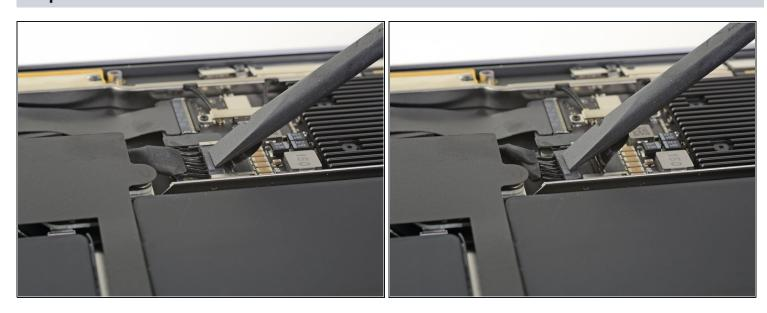
Use a spudger to slide the battery connector parallel to the logic board and out of its socket on the logic board.
