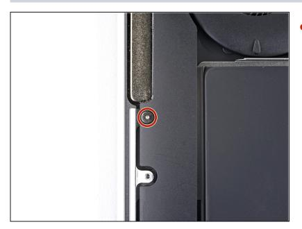
Use a T3 Torx driver to remove the 4.2 mm screw securing the right speaker to the case.
