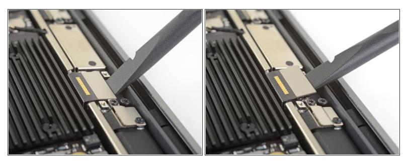
Use the flat end of a spudger to pry the display cable connector straight off of the antenna board to disconnect it.
