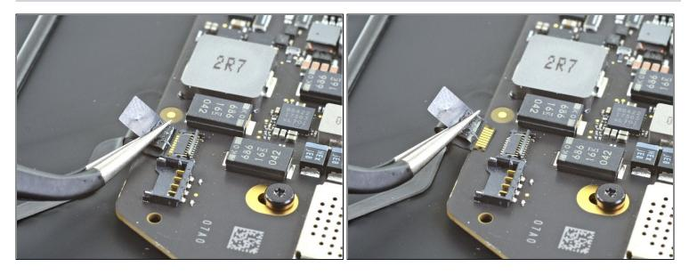
• Slide the microphone cable out of its connector.
