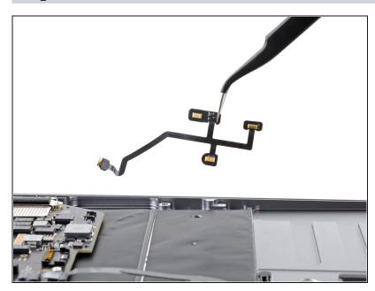
• Remove the microphone array.
