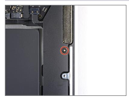
• Use a T3 Torx driver to remove the 4.2 mm screw securing the left speaker to the case.
