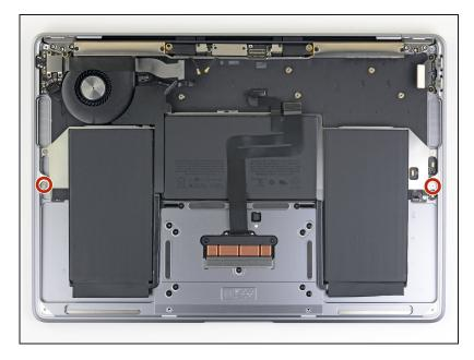
• Use a T3 Torx driver to remove two 2.5 mm screws securing the battery tray to the case.
