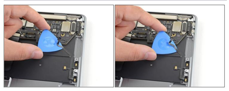
• Slide an opening pick underneath the microphone cable to separate it from the upper case.
