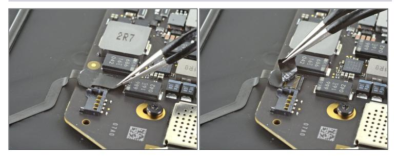
• Use a pair of <u>tweezers</u> to peel back the tape covering the microphone cable connector.
