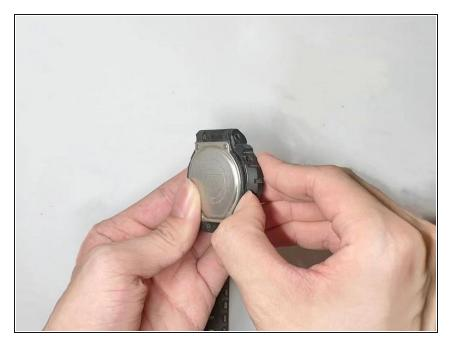
From the bottom of the watch, buckle the case from the main body of the watch by hand.
