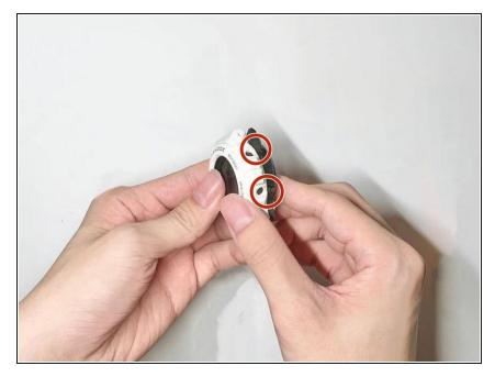
• Align the hole on the side of the case with the button on the watch and put on the new watch case.
