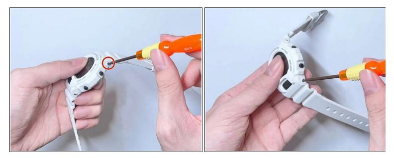
• Screw on the four screws on both sides of the watch.
