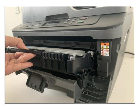
Gently pull the drum unit out of the printer at a slight incline angle.
