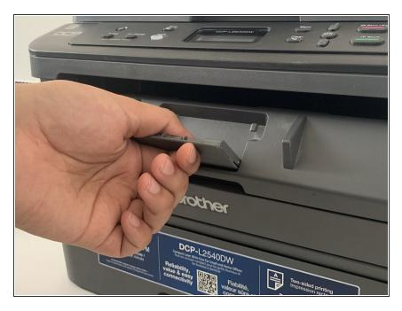
Pull the center paper tray extender to expose the drum unit.
