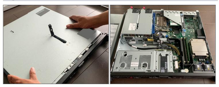
• The top cover will slide backward when the lever is fully extended. Remove the top cover.
