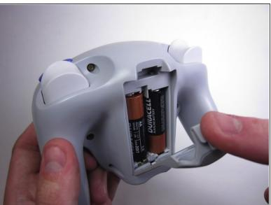
Pull down on the battery cover release lever and pull back to remove the cover.
