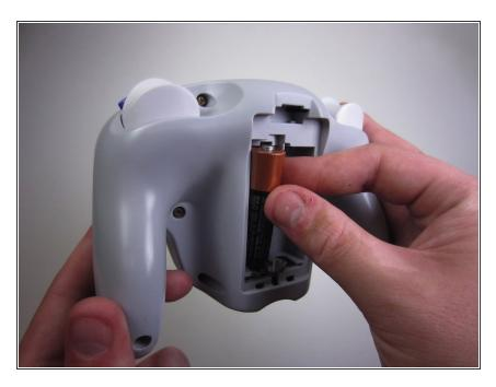
Remove both batteries from the device.
