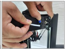
Push and hold the blue lip connected to the tubing and pull out the white PTFE tubing.
