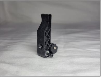
Place the M3 x 8mm screw in the extruder arm making sure that the screw head faces the same direction as the pre-attached screw head.
