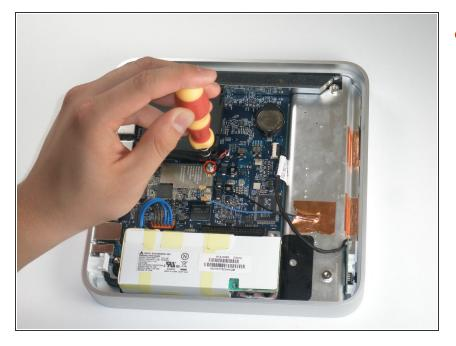
Remove the single T8 Torx screw securing the AirPort card to the logic board.
