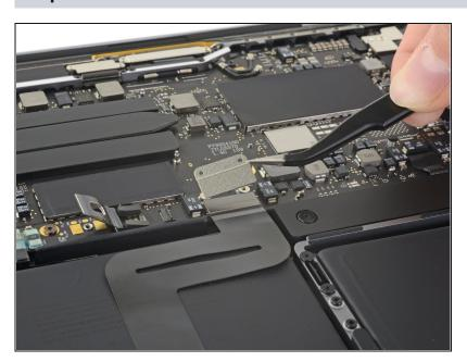
Remove the trackpad cable connector bracket.
