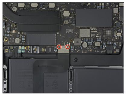
Use a T5 Torx driver to remove the two 1.9 mm screws securing the trackpad cable connector bracket.
