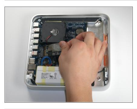
Cautiously lift the AirPort card and pull it straight away. Slide it from its socket on the logic board.
