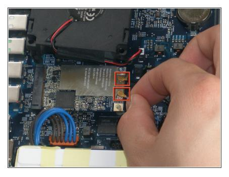
Pry the AirPort antenna cables straight up from their sockets on the logic board.
