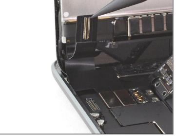
Use the pointed end of a spudger to disconnect the digitizer press connector from the logic board.
