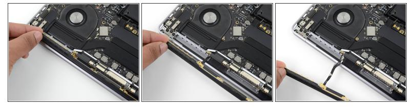
Carefully remove the antenna assembly, while simultaneously feeding the antenna cable bundle out from underneath the heat pipe.
