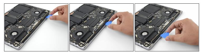
• Use an opening pick to lever out the antenna cable assembly in the areas shown.
